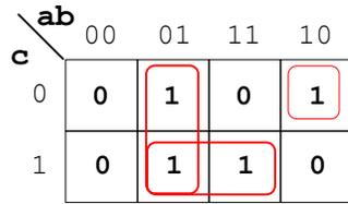
$$f = \bar{a}b + cb + a\bar{b}\bar{c}$$
