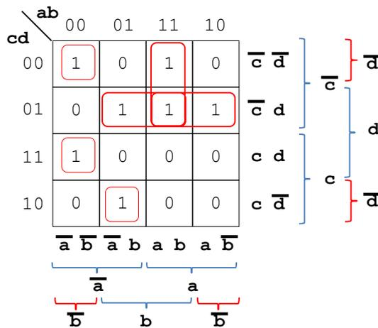
$$f = \bar{a}\bar{b}\bar{c}\bar{d} + \bar{a}\bar{b}cd + \bar{a}bc\bar{d} + ab\bar{c} + a\bar{c}d + b\bar{c}d = \bar{a}\bar{b}(c\oplus d) + \bar{a}bc\bar{d} + ab\bar{c} + \bar{c}d(a+b)$$
